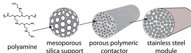
Fig. 1 Schematic of sorbent system in this analysis. The polyamine is located inside the pores of the mesoporous silica support, and the silica support is embedded in the porous polymeric network of the contactor. Contactors are bundled together in modules.
