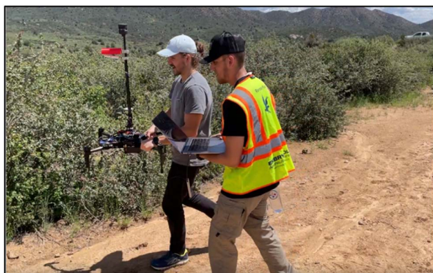
Fig. 19 Calibrating sensors on multirotor aircraft is simplest with two people: one to rotate the vehicle and the other to monitor the flight control software.
