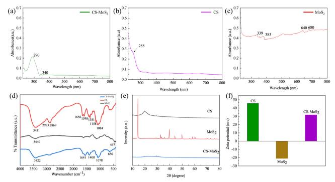
Fig. 5 The UV-Vis absorption (a-c), FTIR (d), XRD (e) and zeta potential (f) spectra of CS, MoS<sub>2</sub> and CS-MoS<sub>2</sub>.
