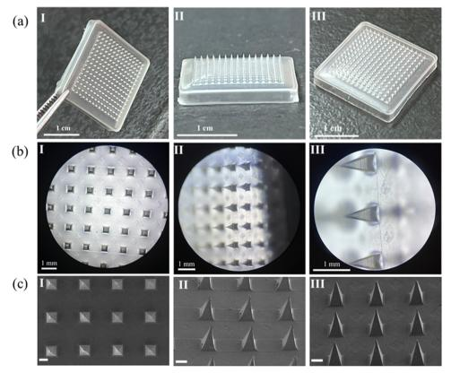
Fig. 3 Morphological characterization images of dissolving HA MNs containing CS-MoS<sub>2</sub>. The direct view of the MNs taken using a mobile phone (a); the shape of the MN tips under an optical microscope (b); the SEM images of the dissolving HA MNs containing CS-MoS2 (c), scale bars: 200 µm.
