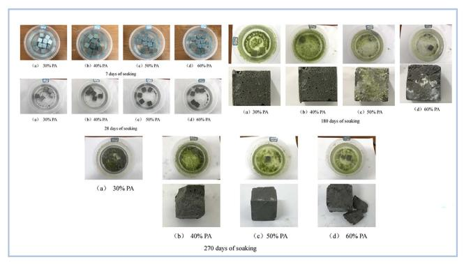
Fig. 16 Evolution of geopolymer specimens different soaking times, Pu et al., Dev. Built Environ., 2022.97
