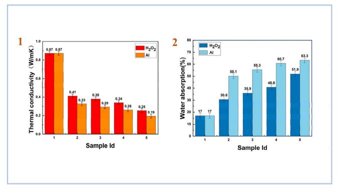
Fig. 13 (1) thermal conductivity of HMNS-FA-phosphate-based porous geopolymers; (2) water absorption (%) of HMNS-FA-phosphate-based porous geopolymers, Yang et al., Minerals, 2023.<sup>83</sup>
