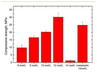
Fig. 7 Compressive strengths of geopolymers synthesized with different concentrations of acid-activator, Wan et al., Gels, 2022.<sup>35</sup>
