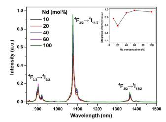
Fig. 2 NIR-II luminescence properties. NIR-II luminescence spectra of a series of Nd-doped Gd<sub>2</sub>O<sub>2</sub>S NPs under 808 nm continuous wave excitation. The concentration of all suspensions is 20 mg  $mL^{-1}$ .
