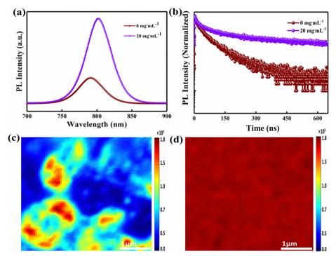
Fig. 5 (a) Steady-state PL spectra and (b) TRPL spectra of control and 20 mg mL<sup>-1</sup>-FAI-based perovskites deposited on the substrate of glass. PL spectral intensity mapping images of (c) control and (d) 20 mg mL<sup>-1</sup>-FAI-based films on the glass substrates.
