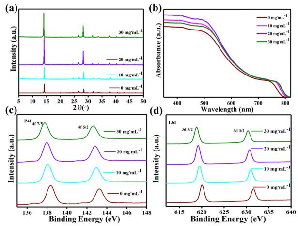
Fig. 4 (a) X-ray diffraction patterns and (b) UV-Vis spectra of the control and FAI-based films with FAI concentrations ranging from 0 mg mL<sup>-1</sup> to  $30 \text{ mg mL}^{-1}$ . XPS spectra of  $0 \text{ mg mL}^{-1}$  to  $30 \text{ mg mL}^{-1}$  FAI-doped perovskites after annealing: (c) Pb 4f and (d) I 3d core spectra of the perovskites with various FAI concentrations.
