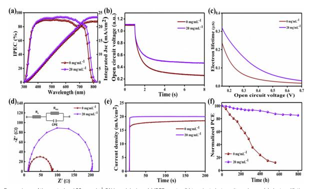
Fig. 7 Comparisons of the control and 20 mg mL $^{-1}$ -FAI based devices: (a) IPCE spectra, (b) transient photo-voltage decays, (c) electron lifetime and  $V_{\rm OC}$ correlation, (d) electrochemical impedance spectroscopy (EIS) with Nyquist plot, (e) stabilized current density at the maximum power point (MPP), and (f) normalized PCE attenuation under 30% relative humidity and 25 °C for about 800 h.
