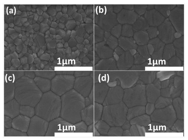
Fig. 3 Surface scanning electron microscopy (SEM) images of the perovskite intermediate adduct modification equipped with varying concentrations of FAI: (a) 0 mg mL $^{-1}$  FAI, (b) 10 mg mL $^{-1}$  FAI, (c) 20 mg mL $^{-1}$  FAI, and (d) 30 mg mL $^{-1}$  FAI.
