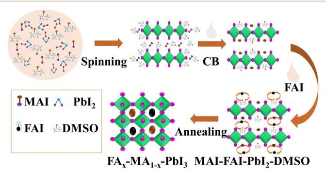
Fig. 1 Schematic of DMSO-FAI molecular interchange to form the FA<sub>x</sub>MA<sub>1-x</sub>PbI<sub>3</sub> perovskite.
