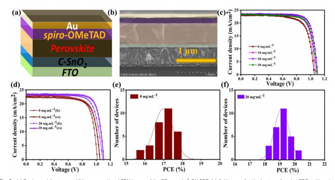
Fig. 6 (a) Device architecture and (b) cross-sectional SEM image of the 20 mg mL<sup>-1</sup>-FAI PSC. (c) J–V curves for the best-performing PSCs with various FAI concentrations. (d) J-V curves of control and 20 mg mL<sup>-1</sup>-FAI treated PSCs with reverse and forward scans. Distribution PCE of (e) 0 mg mL<sup>-1</sup> and (f) 20 mg mL<sup>-1</sup>-FAI treated devices. There are 30 and 28 devices of the statistical distribution of PCEs for control and 20 mg mL<sup>-1</sup>-FAI PSCs.
