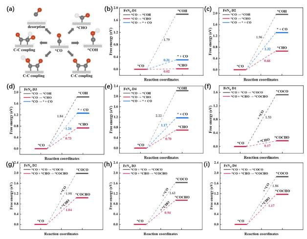
Fig. 4 (a) Schematic diagram of different reaction pathways of the \*CO intermediate. (b-e) Free energy profile of CO desorption and \*CO hydrogenation. (f-i) Comparison of C-C coupling on four FeN<sub>4</sub>-Dx (x = 1, 2, 3, 3 and 4) structures.
