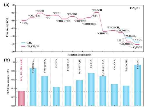
Fig. 5 (a) Reaction free energy profile of  $CO_2$  reduction to  $C_2H_4$  and  $C_2H_5OH$  on the  $FeN_4-D1$  structure. (b) Comparison of the  $FeN_4-D1$  structure with some reported catalysts on the PLS free energy of C<sub>2</sub>H<sub>5</sub>OH.
