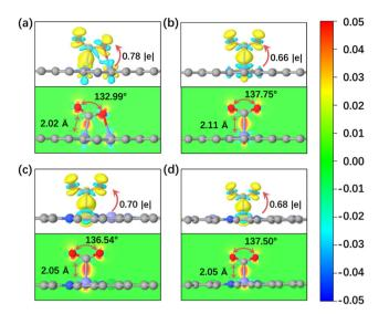
Fig. 2 (a-d) Charge density difference and Bader charge transfer of CO<sub>2</sub> adsorbed on  $FeN_4$ -Dx (x = 1, 2, 3, and 4) (the regions in yellow and cyan represent, respectively, electron accumulation and deletion. The isosurface levels are 0.005 e bohr<sup>-3</sup>).
