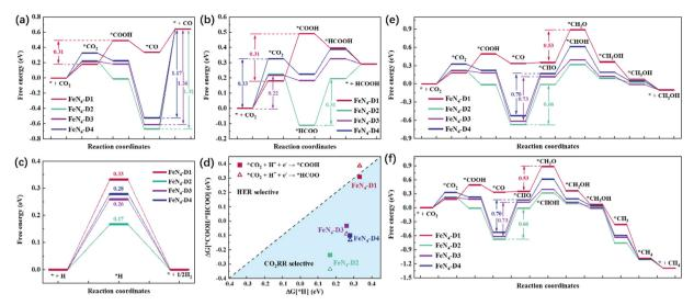
Fig. 3 Reaction free energy profile of  $CO_2$  reduction to CO (a) and HCOOH (b). HER free energy profile (c) and the comparison between the HER and  $CO_2$ RR on the four catalysts (d). Reaction free energy profile of the  $CO_2$ RR to  $CH_3$ OH (e) and  $CH_4$  (f) on  $FeN_4$ -Dx (x = 1, 2, 3, 3 and 4) structures.
