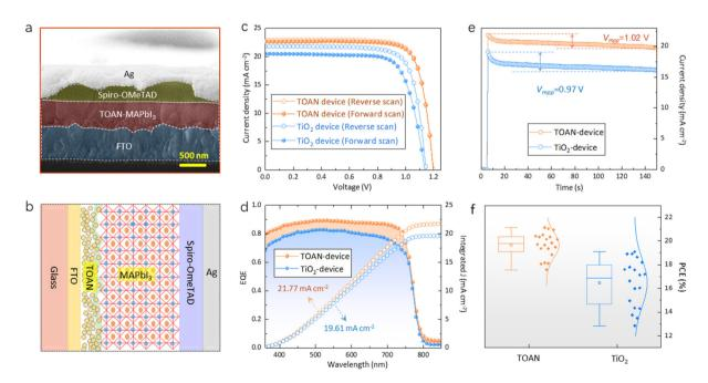
Fig. 5 Device performance. (a) Cross-sectional SEM and (b) schematic structure of the PSCs. (c) J-V curves and (d) EQE spectra of the champion TiO<sub>2</sub> and TOAN devices. (e) The output photocurrent is taken from the maximum power point of the champion devices. (f) PCE distribution of 20 TiO<sub>2</sub> and 20 TOAN devices, respectively.
