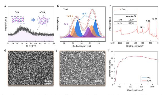
Fig. 1 Construction and characterization of the TOAN ETL. (a) XRD pattern of the ~80 nm a-TaN<sub>x</sub> film deposited on glass. XPS patterns of (b) Ta 4f and (c) a-TaN<sub>x</sub> films. The SEM images of (d) TiO<sub>2</sub> and (e) TOAN layers on FTO substrates. (f) The optical transmittance of the TiO2 and TOAN layers.
