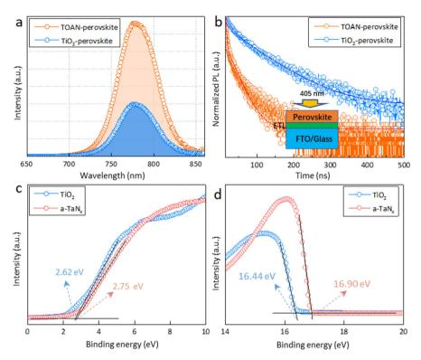
Fig. 4 Carrier transport at the TOAN/perovskite interface. (a) Steady-state PL and (b) TRPL spectra of the TiO2- and TOAN-perovskite films, respectively. (c) The onset and (d) the cutoff of the UPS spectra for the  $TiO_2$  and  $a-TaN_x$  films, respectively.
