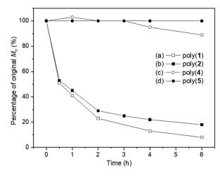
Fig. 6 Plot of original  $M_n$  percentage vs. time, following the degradation of poly(1)  $(M_{n,SEC}=10~000~{\rm g~mol^{-1}}, D_{\rm M}=1.77),^{21}~{\rm poly(2)}~(M_{n,SEC}=5500~{\rm g~mol^{-1}}, D_{\rm M}=1.54),~{\rm poly(4)}~(M_{n,SEC}=6300~{\rm g~mol^{-1}}, D_{\rm M}=1.30)$  and poly(5)  $(M_{n,SEC}=4900~{\rm g~mol^{-1}}, D_{\rm M}=1.16)$  when exposed to UV light ( $\lambda=365~{\rm nm}$ ) for 6 hours, at room temperature, in THF solution.
