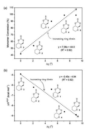
Fig. 3 (a) Plot of  $\Delta\chi$  vs. monomer conversion (b) relationship between  $\Delta\chi$  obtained from XRD data and  $\Delta H_{\rm ROP}$  calculated as a representation of ring strain.
