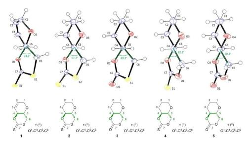
Fig. 2 ORTEP drawings of the crystal structure of 1-5 with thermal ellipsoids at the 50% probability level (see ESI‡). For each crystal structure the  $O-C^4-C^5-C^6$  torsion angle is drawn and highlighted in the accompanying structures below. Single crystals were obtained for each monomer by layering chloroform with n-hexane.
