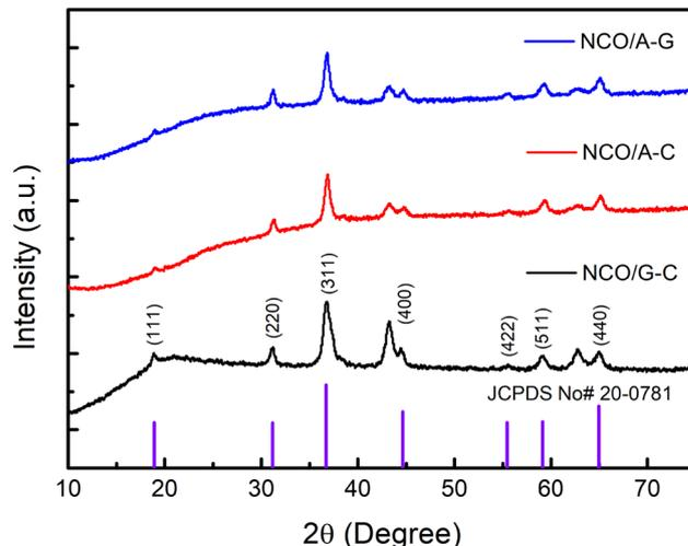
Fig. 2 XRD patterns of the prepared NCO–nucleobase electrode materials.
