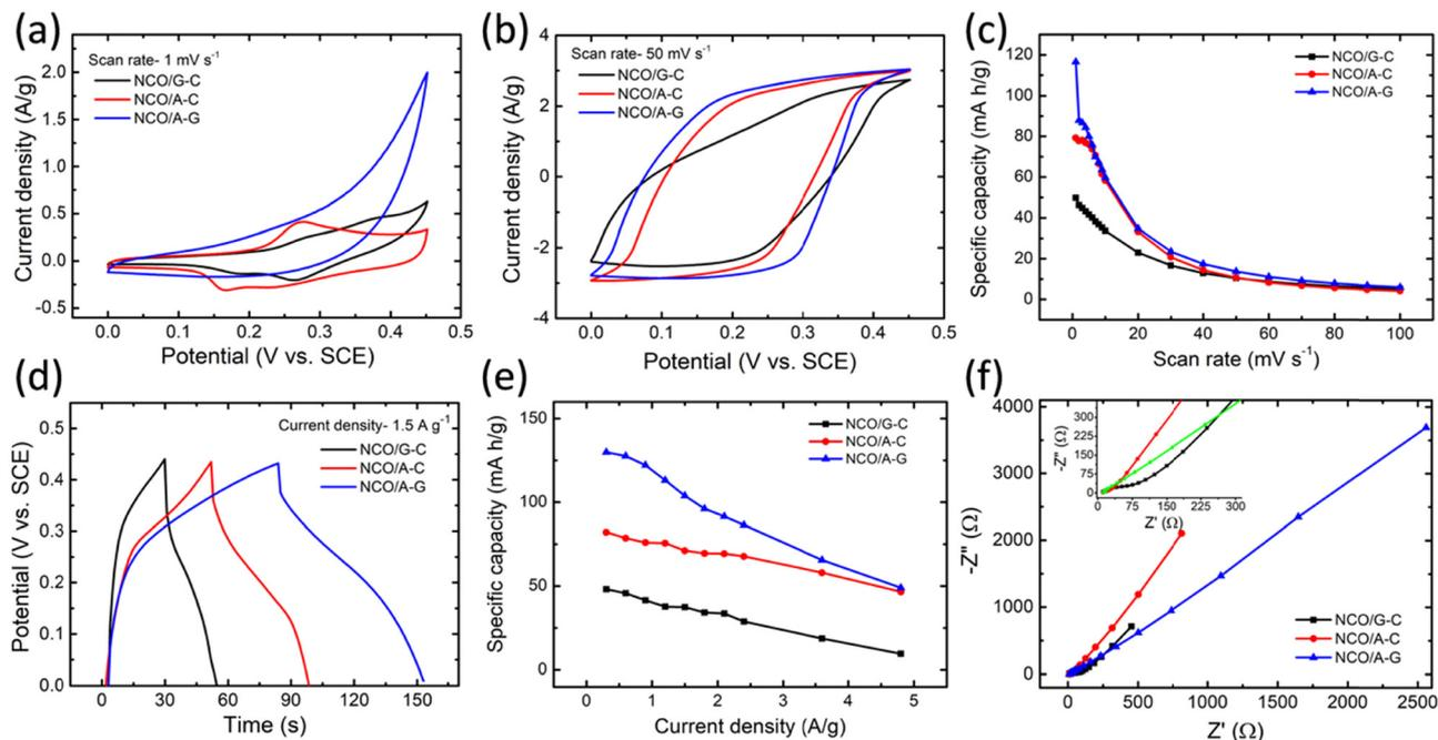
Fig. 5 CV curves of the NCO/G-C, NCO/A-C, and NCO/A-G obtained at the sweep rates of (a)  $1 \text{ mV s}^{-1}$  and (b)  $50 \text{ mV s}^{-1}$ , (c) scan rate dependent specific capacity plot, (d) GCD plots at a current density of  $1.5 \text{ A g}^{-1}$ , (e) the corresponding specific capacity plots at different discharge current densities, and (f) Nyquist plots of all NCO-based electrodes in  $3 \text{ M KOH}$  solution (inset is the magnified view).
