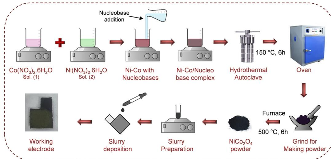
Fig. 1 Schematic representation of the synthesis procedures of NCO–nucleobase complexes and the preparation of the NCO-based working electrode.
