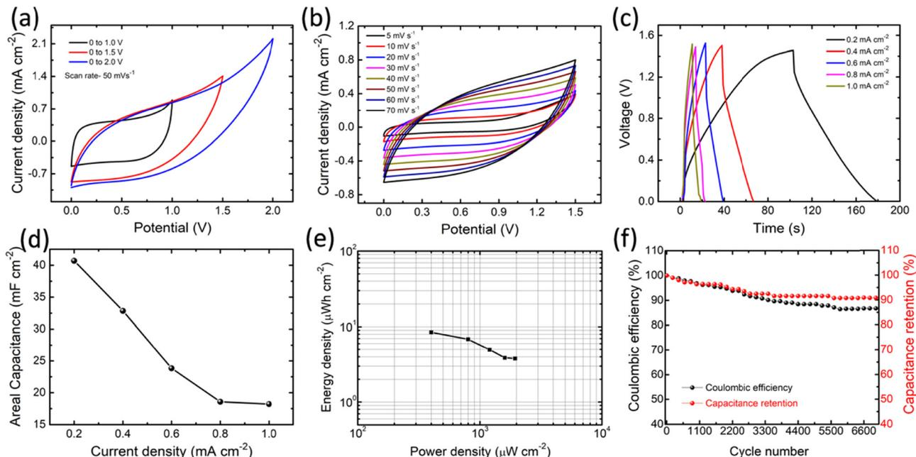
Fig. 6 NCO/A-G-based ASC measurements: CV curves with (a) different potential windows (0–1 V, 0–1.5 V, and 0–2.0 V), (b) scan rates (5–70  $\text{mV s}^{-1}$ ), (c) GCD plots with various current densities (0.2–1.0  $\text{mA cm}^{-2}$ ), (d) the corresponding areal capacitance ( $C_a$ ) at different discharge current densities, (e) Ragone plot, and (f) capacitance retention as a function of charge–discharge cycles.
