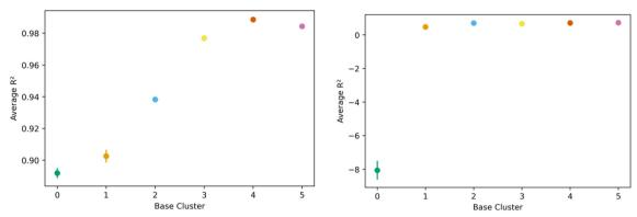
Fig. 10 Task transfer learning performance as average R<sup>2</sup> value as a function of base generic cluster. On the left is transfer from hydrogen at 77 K to hydrogen at 243 K at 100 bar, and mirrors Fig. 7's non-task transfer results. On the right is transfer from hydrogen at 243 K to methane at 298 K. Note the change in scale of the vertical axis.
