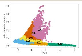
Fig. 3 Standardized adsorption performance for hydrogen at 100 bar and 243 K with respect to each PC. Different clusters clearly occupy different areas of the adsorption space with respect to PC1 and PC2.
