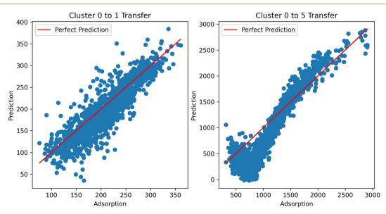
Fig. 11 TL performance using hydrogen adsorption as the source and methane as the target task across clusters. TL from cluster 0 to cluster 1 performs well, but not for cluster 5.
