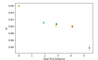
Fig. 5 Example of how transfer model performs in different clusters, using cluster 1 as the base for direct learning. An increase in the PCA distance between clusters leads to lower performance of the resulting model.
