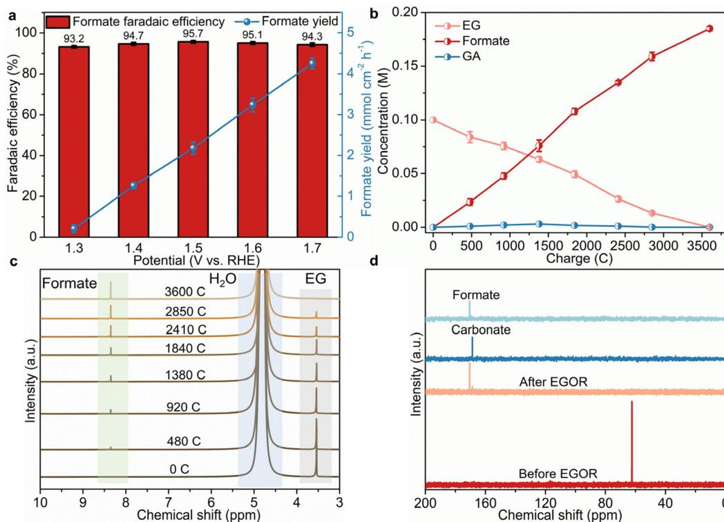
**Fig. 3** (a) faradaic efficiency and yield for formate production of B,Co-NiS from 1.3 to 1.7 V vs. RHE. (b) Charge-dependent concentration of reactants, intermediates, and products. (c)  $^1\text{H}$  NMR spectra of products during the EGOR process. (d)  $^{13}\text{C}$  NMR spectra of initial electrolytes and electrolytes after the EGOR.
