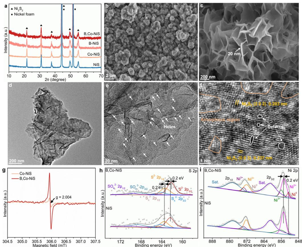
**Fig. 1** (a) XRD patterns of catalysts. (b and c) SEM images of B,Co-NiS. (d and e) TEM images of B,Co-NiS. (f) High-resolution TEM (HRTEM) image of B,Co-NiS. (g) EPR spectra of Co-NiS and B,Co-NiS. XPS spectra for (h) S 2p and (i) Ni 2p of B,Co-NiS and NiS.
