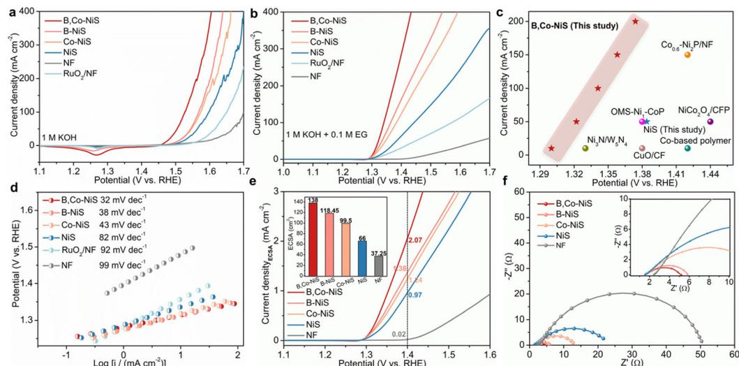
**Fig. 2** (a) OER linear sweep voltammetry (LSV) curves of catalysts. (b) EGOR LSV curves of catalysts. (c) Comparison of B,Co-NiS with state-of-the-art TM-based EGOR catalysts. (d) Tafel plots of electrocatalysts for the EGOR. (e) ECSA normalized EGOR LSV curves, and inset shows the calculated ECSA value of electrocatalysts. (f) EIS Nyquist plots of electrocatalysts, and inset shows an enlarged part of Nyquist plots.
