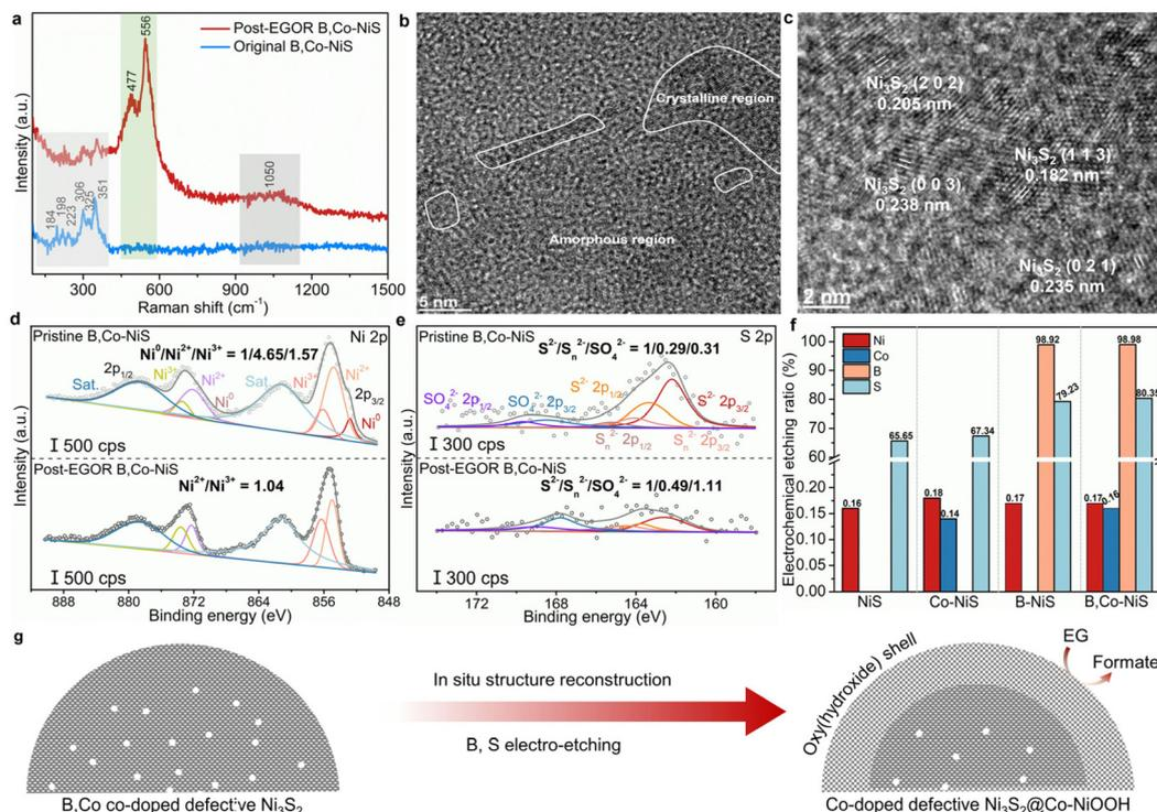
**Fig. 4** (a) Raman spectra of B,Co-NiS before and after the EGOR process. (b) TEM and (c) HRTEM images of B,Co-NiS after the EGOR process. XPS spectra for (d) Ni 2p and (e) S 2p of B,Co-NiS before and after the EGOR process. (f) Ion concentrations in electrolytes of different catalysts after the EGOR process. (g) Scheme of the structural reconstruction of B,Co-NiS during the EGOR.
