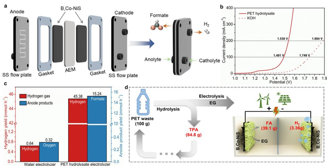
**Fig. 5** (a) The MEA setup for PET hydrolysate and water electrolysis. (b) LSV curves of the PET hydrolysate and water electrolysis. (c) Comparisons of hydrogen gas and anode product yields for PET hydrolysate and water electrolysis systems. (d) Schematic illustration of the PET electro-reforming process and mass flow of products.
