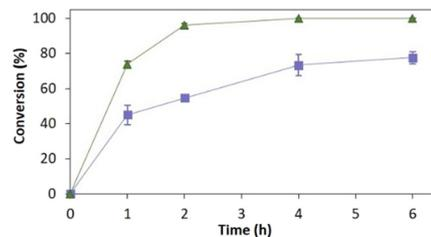
**Fig. 4** Reduction of 2-methyl-*N*-phenylmaleimide **3a** catalysed by immobilised *TsOYE* in MTBE. Conditions: 50 mg *TsOYE*-Celite R-633, 10 mmol **3a**, 1 mmol NADP<sup>+</sup>, 27.7 mmol glucose, 25 mg Na<sub>2</sub>HPO<sub>4</sub>·12H<sub>2</sub>O/Na<sub>2</sub>HPO<sub>3</sub>·5H<sub>2</sub>O, 2 mg GDH-101, MTBE, 1 mL volume, 30 °C. Blue squares: 900 rpm in a thermomixer; green triangles: 180 rpm in an incubator shaker.
