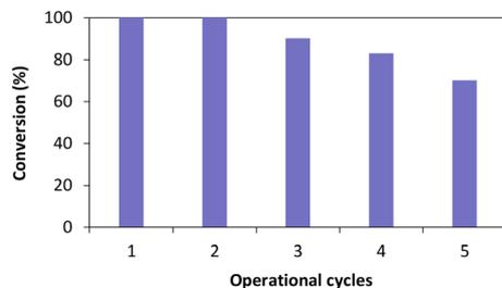
**Fig. 6** Operational cycles of *Ts*OYE immobilised on Celite R-633 for the reduction of cyclohexenone **1a** in MTBE. Conditions: 50 mg *Ts*OYE-Celite R-633, 10 mmol **1a**, 1 mmol NADP<sup>+</sup>, 2 mg GDH-101, 27.7 mmol glucose, 25 mg Na<sub>2</sub>HPO<sub>4</sub>·12H<sub>2</sub>O/Na<sub>2</sub>HPO<sub>3</sub>·5H<sub>2</sub>O, MTBE (1% v/v buffer content), 1 mL volume, 900 rpm, 30 °C, 24 h each cycle.
