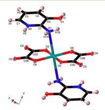
Fig. 2 The Cu coordination in  $(C_5H_7N_2O)_2[Cu(C_2O_4)_2]$  1. The O5 hydroxyl group hydrogen bonds to O3 and the N1 amine. The axial Cu–N bond is 2.711(5) Å.
