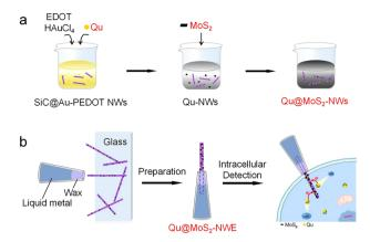
Scheme 1 Illustration of (a) the large-scale synthesis of Qu and MoS<sub>2</sub> cofunctionalized nanowires and (b) the preparation of nanosensors for the electrochemical detection of intracellular hydrogen sulfide.
