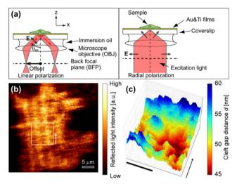
Fig. 3 (a) Schematic illustration of optical paths nearby the sample for lens-imaging-type (LISPM, left) and scanning localized (SLSPM, right) SPRM. (b and c) Representative LISPM (b) and SLSPM (c) images of HEK293 cells cultured on a poly-L-lysine-coated gold surface. Adapted with permission from ref. 57 (Copyright 2014 American Chemical Society).
