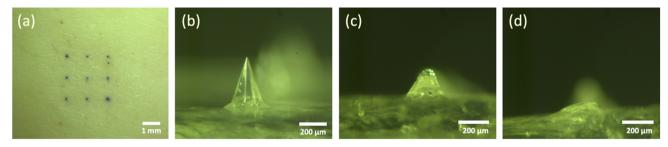
Fig. 3 Representative microscopic images of skin penetration and dissolution tests of empty dMNAs (n = 3). (a) Human abdominal skin ex vivo penetrated with a 5% (w/v) trehalose/pullulan  $3 \times 3$  dMNA. (b)-(d) Microneedle made of 5% (w/v) trehalose/pullulan (b) before skin dissolution and leftover microneedle (c) after 15 minutes and (d) after 30 minutes of skin dissolution.
