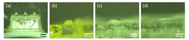
Fig. 4 (a) The fabricated WIV dMNA with 100% of intact microneedles, WIV loaded microneedles after (b) 2 minutes, (c) 5 minutes, and (d) 10 minutes of skin dissolution. The shape of the intact microneedle before dissolution was similar to that in Fig. 3b. Longer dissolution times were not evaluated as the leftover volume after 10 minutes was sufficiently low.
