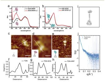
Fig. 2 The characterization of TDN-enzyme conjugations. (a and b) Quantification of SOX-DNA and HRP-DNA conjugation efficiency *via* absorbance spectra. (c-h) AFM images and corresponding measurements of the TDN (c and f), TDN-SOX (d and g) and TDN-HRP(e and h), respectively. Scale bar: 20 nm. (i) Schematic of a TDN-enzyme structure model. (j) Fitting of the experimental SAXS profile for the TDN-enzyme structure model by CRYSOL.
