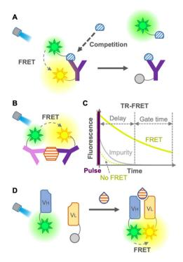
Fig. 2 FRET immunosensors. (A) Scheme of a competitive FRET immunosensor. (B) Scheme of a non-competitive FRET immunosensor. (C) Principle of the TR-FRET immunoassay. Fluorescence from the acceptor (green) and impurity (gray). (D) Scheme of an open sandwich non-competitive immunoassay. "Y" shape: antibody; semicircle: small molecule antigen; hexagon: large molecule antigen; drop shape: large or small molecule antigen; and sun shape: fluorophore.
