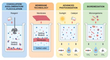
Fig. 6 An overview of microplastic remediation technologies
