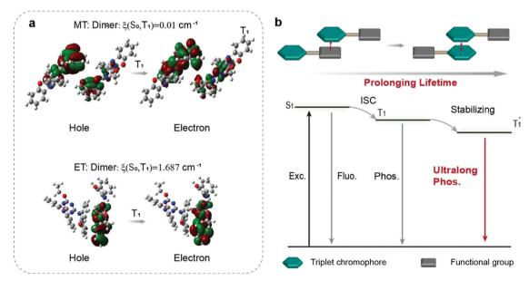
Fig. 4 Proposed mechanism for ultra-long phosphorescence (a). Natural transition orbitals (NTOs) of T1 states for the MT and ET dimer. (b) The mechanism of the different emission behaviours in the compound
