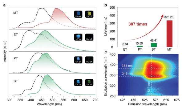
Fig. 2 Photophysical properties of MT, ET, PT and BT in crystals under ambient conditions. (a) Normalized steady-state photoluminescence (dotted lines) and phosphorescence (solid lines) spectra of MT, ET, PT and BT crystals. Insets: Photographs of MT, ET, PT and BT crystals under 365 nm UV light on (left) and off (right). (b) Comparison of phosphorescence lifetimes for MT, ET, PT and BT in crystals. (c) Excitation-phosphorescence emission mapping of the MT crystal.
