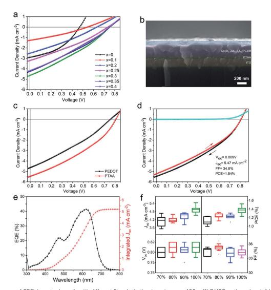
Fig. 4 (a) J-V curves of CBSI-based solar cells with different Sb substitution by using pure 100 vol% DMSO as the solvent. (b) Cross-sectional SEM image of the CBSI-3 solar cell by using PTAA as the HTL. (c) J-V curves of the CBSI-3 solar cells with PEDOT or PTAA as the HTL. (d) J-V and (e) EQE curves of the champion CBSI-3 solar cell. (f) Statistic variations of CBSI-3 devices fabricated by using solvents with different DMSO volume ratios.
