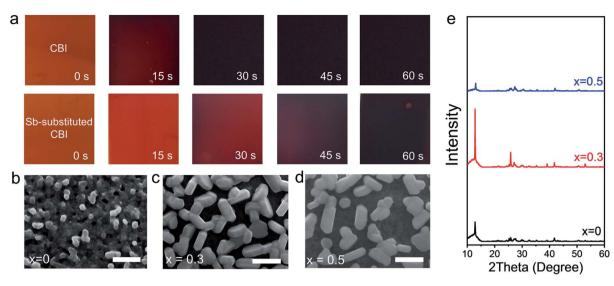
Fig. 1 (a) Photographs of CsBi<sub>3</sub>I<sub>10</sub> (CBI) and Cs(Bi<sub>0.7</sub>Sb<sub>0.3</sub>)<sub>3</sub>I<sub>10</sub> (CBSI-3) films with different thermal annealing duration. SEM images of (b) CBI, (c) CBSI-3, and (d) CBSI-5 films, the scale bar corresponds to 500 nm. (e) XRD patterns of CBI (x = 0), CBSI-3 (x = 0.3), and CBSI-5 (x = 0.5) films. (All films illustrated here are synthesized from DMF/DMSO mixed solvent with the volume ratio of 9:1).
