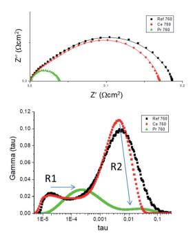
Equivalent circuit and DRT fittings at 760 °C.
