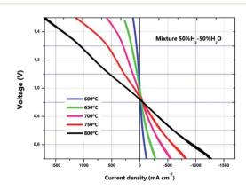
Fig. 7 Current density (j) versus voltage (V) in both fuel cell and electrolysis mode performed at temperatures between 600 and  $800\,^{\circ}\text{C}$  for the manganese infiltrated cell.
