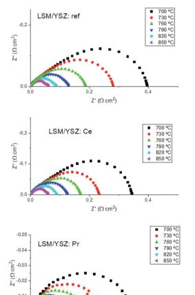
Fig. 3 Impedance plots at different temperatures for standard, Ceinfiltrated and Pr-infiltrated LSM/YSZ symmetrical cells at different temperatures
