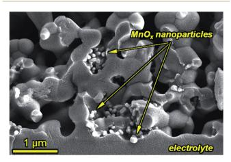
Fig. 2 SEM image of manganese oxide infiltrated nanoparticles in the active region of the cathode. Secondary electron image of a fractured electrode-electrolyte interface ( $E_e = 5 \text{ keV}$ ).
