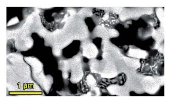
Fig. 6 (Up) Chronoamperometry experiment at 0.7 V and 700  $^{\circ}$ C for one day; (down) SEM images showing the microstructure of the Pr<sub>6</sub>O<sub>11</sub> infiltrated into LSM–YSZ electrodes after all the electrochemical measurements (total period of about 100 hours mostly at 800  $^{\circ}$ C). Backscattered images were obtained on infiltrated and polished samples at  $E_{\rm e}=10$  keV.
