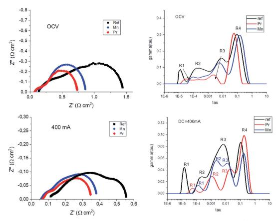
Nyquist plots (left) and DRT analysis (right) performed under OCV conditions and under DC =  $400 \text{ mA cm}^{-2}$  (SOFC mode).
