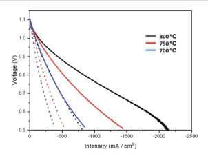
Fig. 5 Comparison between a standard non impregnated cell (dotted line) and a cell impregnated with 2.5 wt%  $\rm Pr_6O_{11}$  (continuous thick line) at temperatures of 700 °C, 750 °C and 800 °C.
