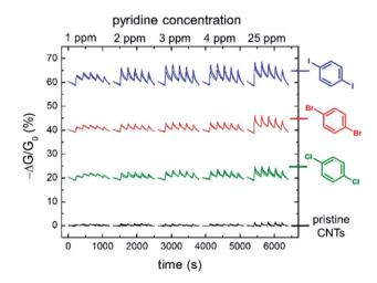
Fig. 37 Conductance response of chemiresistive gas sensors containing different dihaloaryl XB selectors in the repeating presence of increasing concentrations of pyridine in  $N_2$  carrier gas. For clarity the relative conductance responses are offset by 20%. Reproduced with permission from ref. 171 copyright 2016 American Chemical Society.
