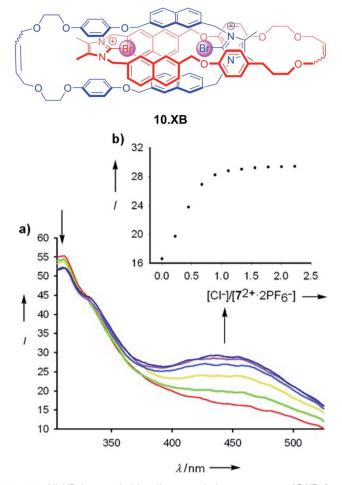
Fig. 13 All-XB bromo-imidazolium-napthalene catenane 10.XB for fluorescent halide sensing. (a) Emission spectra of 10  $\mu\text{M}$  10.XB upon addition of Cl $^-$  in ACN. (b) The corresponding response isotherm at 445 nm. Reproduced with permission from ref. 122 copyright 2011 Wiley.
