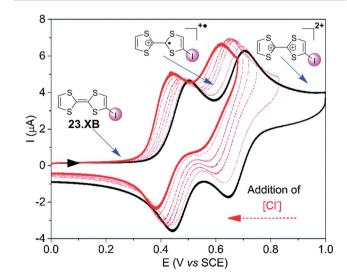
Fig. 24 Chemical structure of iodo-TTF 23.XB and its corresponding CV in DMF in the absence (black) and presence (red) of increasing concentrations of Cl<sup>-</sup>. Depicted are also the different redox states at different potentials (structures and blue arrows). Adapted from ref. 138 with permission from the PCCP Owner Societies.
