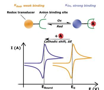
Fig. 20 Schematic depiction of voltammetric anion sensing at a redox active anion receptor. Receptor oxidation/reduction is reflected in anion binding enhancement/decrease. In the presence of a binding anion the half-wave potential is perturbed cathodically, whereby the shift magnitude is directly proportional to the ratio of anion binding constants to the different receptor oxidation states:  $\Delta E \propto K_{\rm Ox}/K_{\rm Red}$ .
