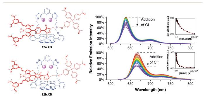
Fig. 15 Fluorescence response of  $1 \,\mu\text{M}$  XB BODIPY-containing strapped porphyrin rotaxanes 12a.XB (top) and 12b.XB (bottom) towards Cl<sup>-</sup> in acetone. The insets show the corresponding response isotherms, highlighting stronger binding and a larger response for the more polarised, perfluorobenzene-containing 12b.XB. Reproduced from ref. 79 under the terms of the CC BY license.
