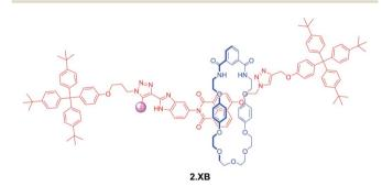
Fig. 7 XB [2]rotaxane molecular shuttle 2.XB for colorimetric anion sensing in CHCl<sub>3</sub>. Only in the presence of a coordinating Cl<sup>-</sup> anion as well as acid-induced protonation of the benzimidazole does the macrocycle shuttle towards the XB anion binding site, resulting in a disruption of the hydroquinone-NDI charge-transfer interaction and a concomitant loss of colour.
