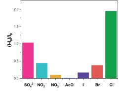
Fig. 10 Relative emission intensity increase of 10  $\mu M$  tetraphenylethene AIE anion sensor 5.XB in the presence of 10 equiv. of various anions in THF. Reproduced from ref. 100 under the terms of the CC BY license
