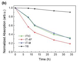
Fig. 6 (a) Plots of the NFA conversion ratio calculated from 1H NMR spectra as a function of reaction time with an ethanolamine: acceptor ratio of 4:1 at room temperature; (b) plots of the normalized absorption intensity of the main peak as a function of reaction time. Reproduced from ref. 45 with permission from the American Chemical Society, copyright [2020].
