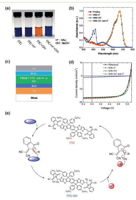
Fig. 5 (a) Image, and (b) the absorbance of four different ITIC solutions: pristine, and with the addition of  $H^+$ ,  $OH^-$ , and both  $OH^-$  and  $H^+$ ; (c) device structure; (d) J-V characteristics of devices with active layers having acid or base additives; (e) scheme of the reversible reaction of ITIC under acidic and basic conditions. Reproduced from ref. 44 with permission from the American Chemical Society, copyright [2019].
