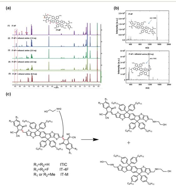
Fig. 4 (a) In situ 1H NMR spectra of pristine IT-4F and IT-4F after adding different equivalents of ethanolamine; (b) the mass spectra of pristine IT-4F and IT-4F after adding 8.0 eq. ethanol amine, respectively. The detection was operated in negative ion mode; (c) reaction scheme of NFA of ITIC and ethanolamine. Reproduced from ref. 43 with permission from the Nature Publishing Group, copyright [2020].
