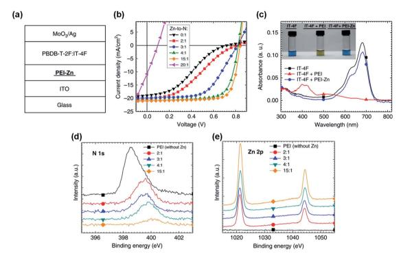
Fig. 13 (a) Structure of OSC devices; (b) J-V characteristics of the devices with PEI-Zn ETL containing different Zn-to-N mole ratios; (c) absorption spectra of three solutions: IT-4F, IT-4F mixed with PEI, and IT-4F mixed with PEI-Zn solution. The inset shows the pictures of the three solutions; (d and e) XPS spectra of the PEI-Zn films containing different Zn-to-N ratios: e N 1s; f Zn 2p. Reproduced from ref. 43 with permission from the Nature Publishing Group, copyright [2020].
