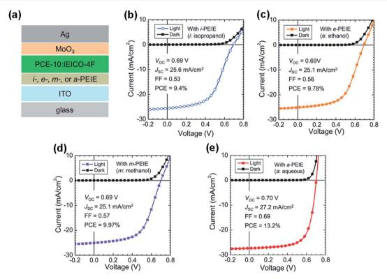
Fig. 12 (a) Device structure of OSCs: i-, e-, m-, and a-PEIE denote PEIE processed from isopropyl alcohol, ethanol, methanol, and aqueous solutions, respectively; (b-e) J-V characteristics of the non-fullerene OSCs with different interfacial layers: (b) with i-PEIE; (c) with e-PEIE; (d) with m-PEIE; (e) with a-PEIE. Reproduced from ref. 47 with permission from the Wiley, copyright [2019].
