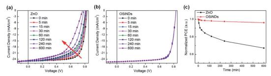
Fig. 17 (a) With ZnO ETL; (b) with OSiND ETL; (c) the evolution of PCEs for the devices under continuous illumination. Reproduced from ref. 86 with permission with Wiley, copyright [2020].
