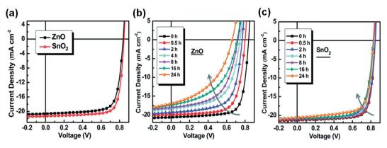
Fig. 23 (a) J-V characteristics; (b and c) evolution of the J-V characteristics of cells under continuous AM1.5 G illumination: (b) with the ZnO ETL and (c) the SnO<sub>2</sub> ETL, respectively. Reproduced from ref. 46 with permission from the Royal Society of Chemistry, copyright [2019].
