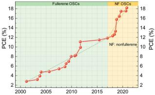
Fig. 1 Power conversion efficiency evolution of organic solar cells (data extracted from the NREL Best Research-Cell Efficiency Chart).<sup>31</sup> The dashed line is a guide for the eye to show the approximate slop of efficiency increase.
