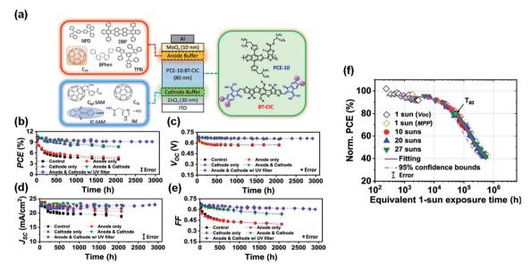
Fig. 22 (a) Schematic of the device and molecular structures of the cathode and anode buffer materials; (b) PCE; (c)  $V_{OC}$ ; (d)  $J_{SC}$  and (e) FF plotted vs. aging time under 1-sun AM1.5G illumination for 3000 h with different device architectures; (f) normalized PCE plotted vs. the equivalent 1-sun exposure time. Reproduced from ref. 94 with permission from the Nature Publishing Group, copyright [2021].
