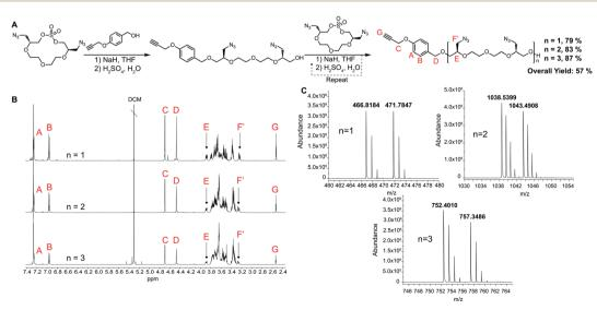
Fig. 2 Synthesis of AzMCS polymers. (A) Synthesis of propargyl hexaazide polymer, (B) purified NMR of each ring-opening step, and (C) mass spectrum of each chain extension (NH<sub>4</sub><sup>+</sup> and Na<sup>+</sup> adducts).
