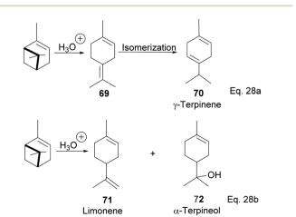
Scheme 24 Acid-catalyzed hydration of  $\alpha\text{-pinene}$  to monocyclic terpenoid derivatives.
