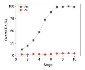
Fig. 8 Effect of ion flotation stage on the recovery efficiency of Pb and Zn. Conditions:  $[Zn]_i=22.5 \text{ mmol L}^{-1}$ ,  $[Pb]_i=3.5 \text{ mmol L}^{-1}$ ,  $[CTAB]_{total}=9 \text{ mmol L}^{-1}$  (0.9 mmol L<sup>-1</sup> per stage),  $t_{total}=50 \text{ min (5 min per stage)}$  [EtOH] = 0.5% (v/v), V=50 mL, flowrate = 25 mL min<sup>-1</sup>.
