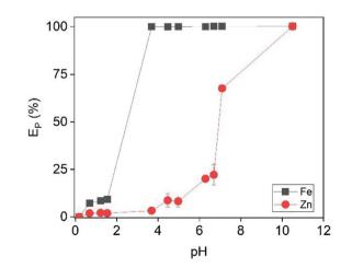
Fig. 9 Effect of pH on the precipitation efficiency of Fe and Zn. Conditions:  $[Zn]_i = 22 \text{ mmol L}^{-1}$ ,  $[Fe]_i = 500 \text{ mmol L}^{-1}$ .
