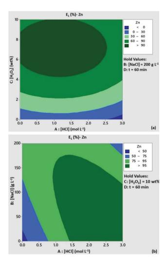
Fig. 3 Contour plots of Zn leaching efficiency as a function of (a) [HCl]/[H<sub>2</sub>O<sub>2</sub>] and (b) [HCl]/[NaCl]. Conditions: L/S = 10 mL  $g^{-1}$ , T=80~C, t=60 min and (a) [NaCl] = 200 g L $^{-1}$ , (b) [H<sub>2</sub>O<sub>2</sub>] = 10 wt%.
