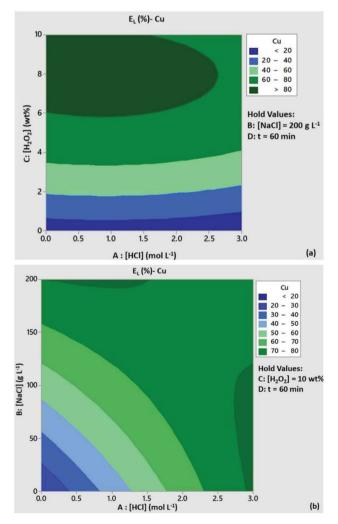
Fig. 2 Contour plots of Cu leaching efficiency as a function of (a) [HCI]/[H<sub>2</sub>O<sub>2</sub>] and (b) [HCI]/[NaCI]. Conditions: L/S = 10 mL g<sup>-1</sup>, T =80 °C, t = 60 min and (a) [NaCl] = 200 g L<sup>-1</sup>, (b) [H<sub>2</sub>O<sub>2</sub>] = 10 wt%.
