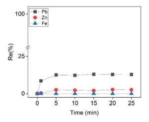
Fig. 7 Effect of ion flotation time on the recovery efficiency of Zn, Pb and Fe from the PLS after the cementation step. Conditions: [CTAB] = 0.9 mmol L $^{-1}$ , [Zn]<sub>i</sub>= 22.5 mmol L $^{-1}$ , [Pb]<sub>i</sub> = 3.5 mmol L $^{-1}$ , [Fe]<sub>i</sub> = 500 mmol L $^{-1}$ , [EtOH] = 0.5% (v/v), V = 50 mL, flowrate = 25 mL min $^{-1}$ .
