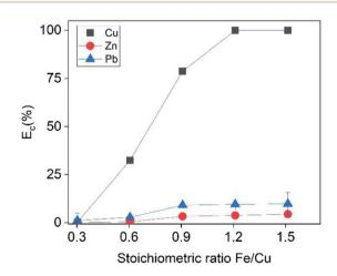
Fig. 5 Cementation efficiency of Cu as a function of the stoichiometric ratio Fe/Cu. Conditions: t=30 min,  $[Cu]_1=500$  mmol  $L^{-1}$ ,  $[Zn]_1=23$  mmol  $L^{-1}$ ,  $[Pb]_1=23$  mmol  $L^{-1}$ .
