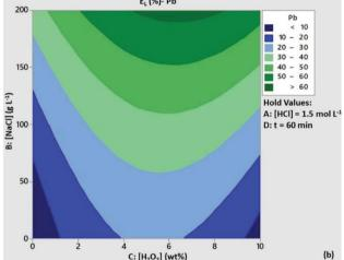
Fig. 4 Contour plots of Pb leaching efficiency as a function of (a) [HCl]/[NaCl] and (b) [H<sub>2</sub>O<sub>2</sub>]/[NaCl]. Conditions: L/S = 10 mL g<sup>-1</sup>, T = 80 °C, t = 60 min and (a) [H<sub>2</sub>O<sub>2</sub>l] = 10 wt%, (b) [HCl] = 1.5 mol L<sup>-1</sup>.
