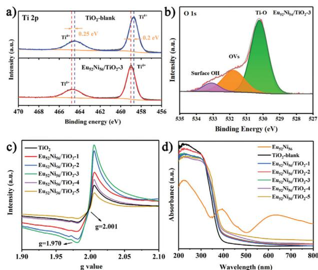
**Fig. 2** (a) Ti 2p XPS profiles of  $\text{TiO}_2$ -blank and  $\text{Eu}_{52}\text{Ni}_{56}/\text{TiO}_2$ -3. (b) O 1s XPS profile of  $\text{Eu}_{52}\text{Ni}_{56}/\text{TiO}_2$ -3. (c) EPR profiles of  $\text{TiO}_2$ -blank and  $\text{Eu}_{52}\text{Ni}_{56}/\text{TiO}_2$ -1, 2, 3, 4, 5. (d) UV-vis DRS profiles of the  $\text{Eu}_{52}\text{Ni}_{56}$  cluster,  $\text{TiO}_2$ -blank, and  $\text{Eu}_{52}\text{Ni}_{56}/\text{TiO}_2$ -1, 2, 3, 4, 5.
