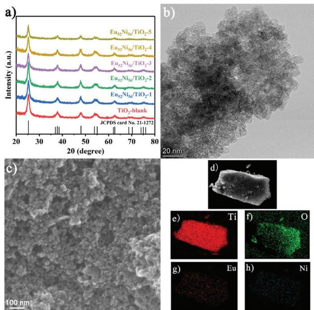
**Fig. 1** (a) PXRD patterns of  $\text{TiO}_2$ -blank and  $\text{Eu}_{52}\text{Ni}_{56}/\text{TiO}_2$ -1, 2, 3, 4, 5. (b) TEM profile of  $\text{Eu}_{52}\text{Ni}_{56}/\text{TiO}_2$ -3. (c) SEM profile of  $\text{Eu}_{52}\text{Ni}_{56}/\text{TiO}_2$ -3. (d–h) Selected area SEM profile of  $\text{Eu}_{52}\text{Ni}_{56}/\text{TiO}_2$ -3, and corresponding EDX elemental mappings of Ti, O, Eu, and Ni.
