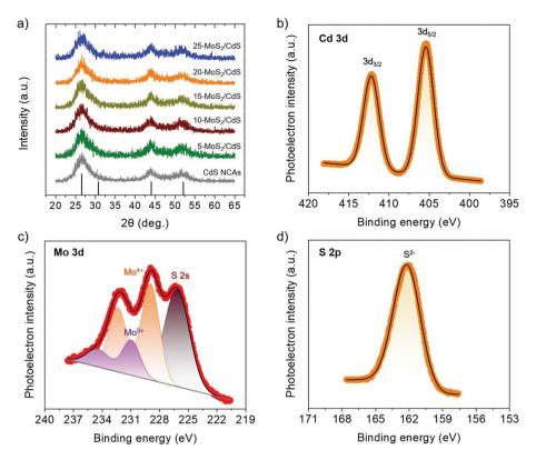
Fig. 1 (a) XRD plots for the mesoporous CdS and MoS<sub>2</sub>/CdS NCAs. The standard diffraction data of the zinc blende CdS according to the JCPDS card no. 42-1411 are also shown (black bars). (b-d) Typical XPS core-level spectra of the Cd 3d (b), Mo 3d (c) and S 2p (d) region for the 20-MoS<sub>2</sub>/ CdS catalyst.
