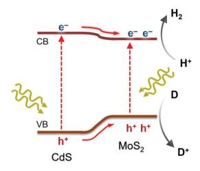
Scheme 1 Expected charge transfer during photocatalytic H<sub>2</sub> production on mesoporous MoS<sub>2</sub>/CdS NCAs under visible light excitation.
