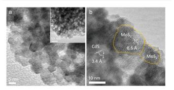
Fig. 2 Representative (a) TEM and (b) HRTEM images of the 20-MoS<sub>2</sub>/ CdS NCAs catalyst.
