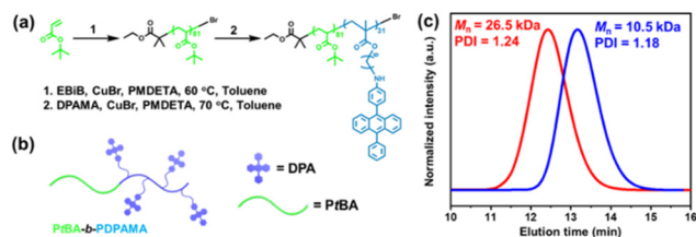
Fig. 1 (a) Polymerization route of the PtBA- b -PDPAMA diblock copolymer. (b) Schematic illustrations of the PtBA- b -PDPAMA diblock copolymer. (c) GPC traces of the PtBA homopolymer (blue) and PtBA- b -PDPAMA diblock copolymer (red).
