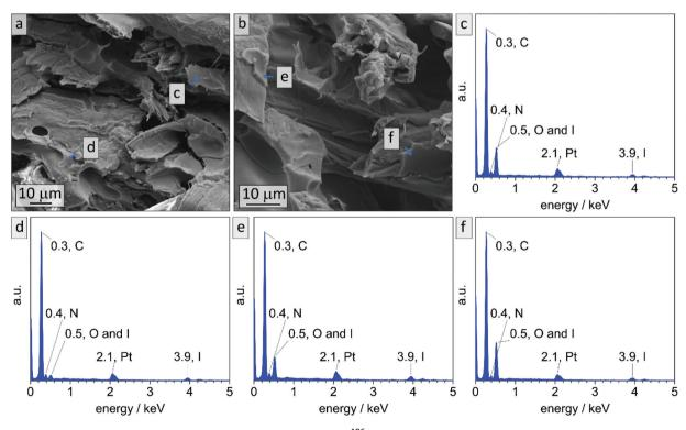
Fig. 10 EDS data collected on composite sample made of Pl<sub>35</sub>-b-P2VP<sub>65</sub><sup>186</sup> on cellulose substrate via vertical deposition after stabilization with DIB. (a and b) Cross-sectional SEM images and exemplary locations of EDS point spectra (c-f) are marked.
