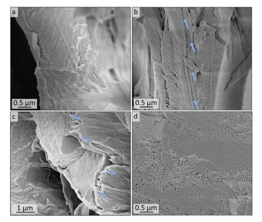
Fig. 9 SEM analysis of the (a and b) cross-sections of untreated and (c and d) ozone treated composite material (sample Cs10) using Pl<sub>35</sub>-b- ${\sf P2VP_{65}}^{\sf 186}$  on Munktell cellulose-based filter discs. Blue arrows indicate cellulose fibers.
