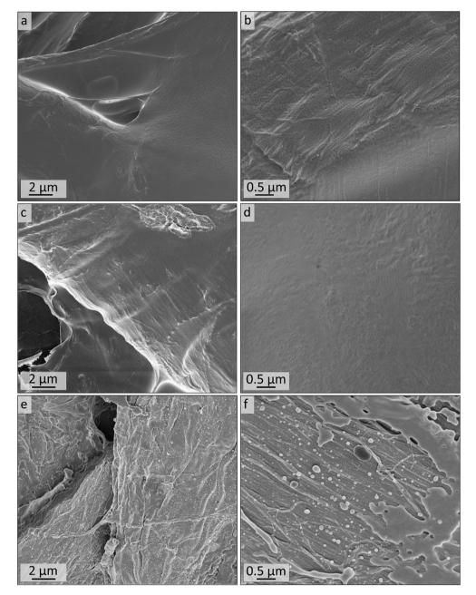
Fig. 8 SEM analysis of (a and b) the surface of untreated and (c-f) ozone treated composite material using  $Pl_{35}$ -b-P2VP<sub>65</sub><sup>186</sup> on Munktell cellulosebased filter discs with increasing magnifications. (c) and (d) show the surfaces of the ozone-treated sample Cs10 (DIB-stabilized), (e) and (f) show surfaces of sample C10 (not stabilized).
