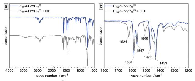
Fig. 4 Analysis of untreated film ( $Pl_{28}$ -b- $P2VP_{72}^{63}$ , blue) and DIB-crosslinked film (gray) by ATR-FTIR transmission spectra. (a) overview, whole spectrum, (b) partial spectrum with changes in P2VP signals.
