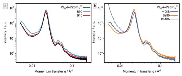
Fig. 7 SAXS of bulk polymer Pl<sub>28</sub>-b-P2VP<sub>72</sub><sup>63</sup> before and after ozone treatment. (a) non-stabilized (Pl<sub>28</sub>-b-P2VP<sub>72</sub><sup>63</sup>) and ozone treated samples B90 and B10. (b) DIB-stabilized (+DIB) and ozone treated samples Bs90 and Bs10b.
