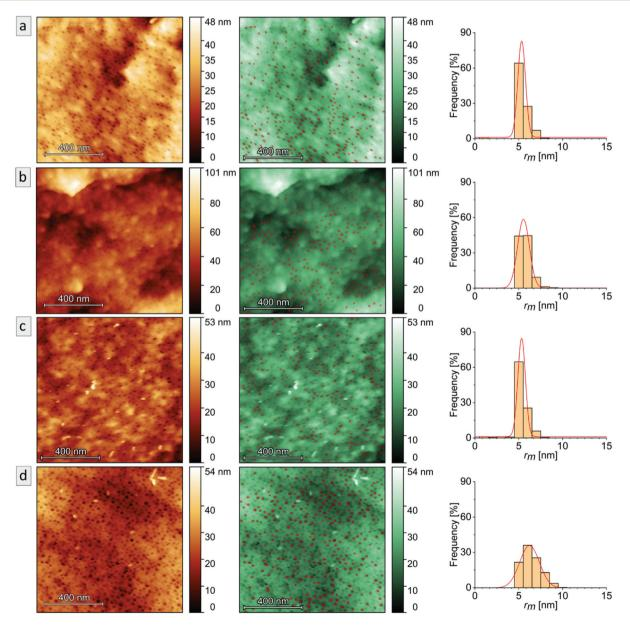
Fig. 6 AFM images (left, in copper), AFM images masked pores (middle, in green) and the respective histograms (right) of the maximum inscribed radius  $r_{\rm m}$  with a Gaussian fit (red curve) of each sample: (a) Bs90, (b) B10, (c) Bs10a and (d) Bs10b. All AFM images were obtained in air at 25 °C.
