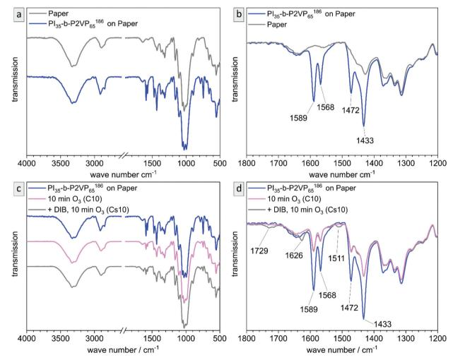
Fig. 11 ATR-FTIR transmission spectra of (a) blank paper and polymer coated paper ( $Pl_{35}$ -b- $P2VP_{65}^{186}$ ) via vertical deposition), (b) partial spectrum of polymer signals of (a). (c) polymer-coated paper ( $Pl_{35}$ -b- $P2VP_{65}^{186}$ ) before and after treating with ozone for 10 min, red curve without DIB-stabilization and blue curve with DIB-stabilization and (d) partial spectrum of polymer signals of (c). All IR-spectra are normalized to the most intensive peak (paper).
