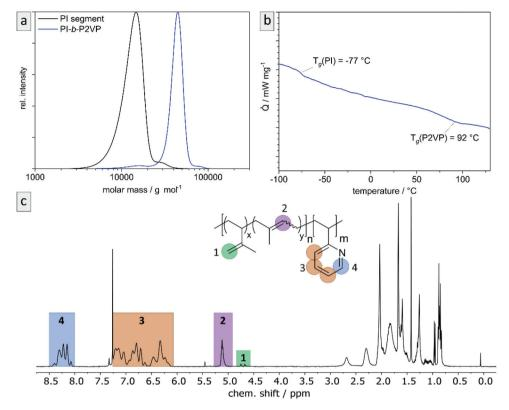
Fig. 1 Exemplary characterization of Pl<sub>28</sub>-b-P2VP<sub>72</sub><sup>63</sup> using (a) SEC to determine relative molar masses (vs. PS-standard) and molar mass distributions, (b) thermograms by DSC measurements to determine glass transition temperatures, and (c) <sup>1</sup>H NMR spectrum in CDCl<sub>3</sub> to determine chemical composition of BCP and microstructure composition of polyisoprene moieties. For evaluated data see Table 1.
