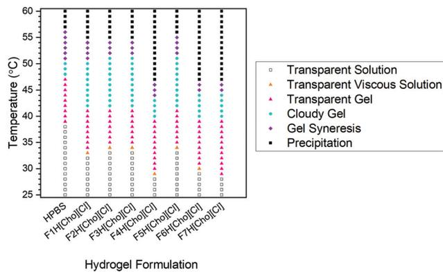
**Fig. 5** Visual state of FITC-IgG in HPBS and hydrogel-IL (2 w/w% OBD) formulations, over the temperature range from 25 to 60 °C. White squares correspond to transparent and runny solution, orange triangles indicate transparent viscous solutions. Pink triangles and blue circles indicate transparent and cloudy stable hydrogels; purple diamonds show gel syneresis, and black squares indicate precipitation.
