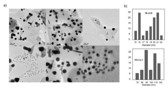
Fig. 9 Characterization of the synthesized AuNPs-CALB-pH4.5 hybrid. (a) TEM images. (b) Nanoparticles size distribution.
