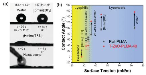
Fig. 3 (a) Contact angles of water, [Bmim][BF<sub>4</sub>], [Hmim][TFSI], and hexadecane on T-ZnO/PLMA-40. (b) Contact angles of liquids on T-ZnO/PLMA-40 and on smooth PLMA versus surface tension. Arrows indicate the wettability amplification from smooth surface to the high-roughness hybrid surface.
