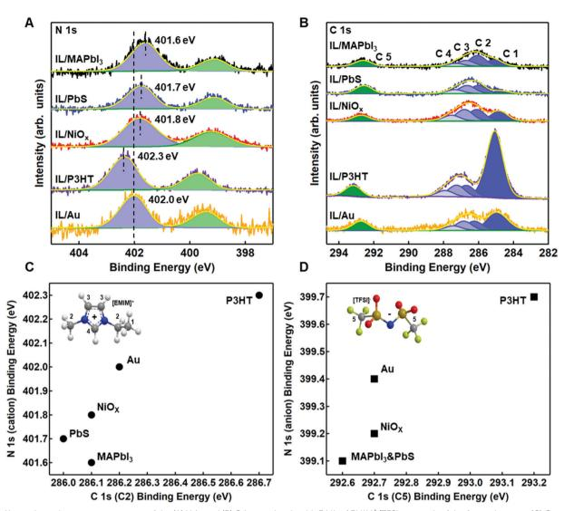
Fig. 4 X-ray photoelectron spectroscopy of the (A) N 1s and (B) C 1s core levels with 3 ML of EMIM\*/TFSI on each of the four substrates. (C) Correlation of the binding energy positions for the C2 carbon on the imidazolium cation, relative to the nitrogen signal and (D) correlation of the binding energy positions for the C5 carbon on the anion imide, relative to the nitrogen signal on each of the substrates. Insets show the labelled carbons for EMIM<sup>+</sup> and TESI referenced in the text
