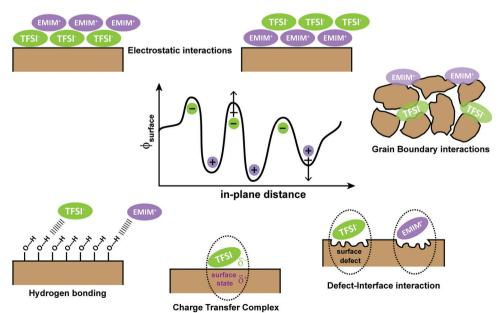
Fig. 1 Schematic of possible nanoscale interactions that can contribute to localized changes in the surface potential ( $\phi_{surface}$ ) at semiconductor/ionic liquid interfaces using EMIM+ (1-ethyl-3-methylimidazolium) and TFSI- (bis(trifluoromethylsulfonyl)-imide) ionic liquid as a model.
