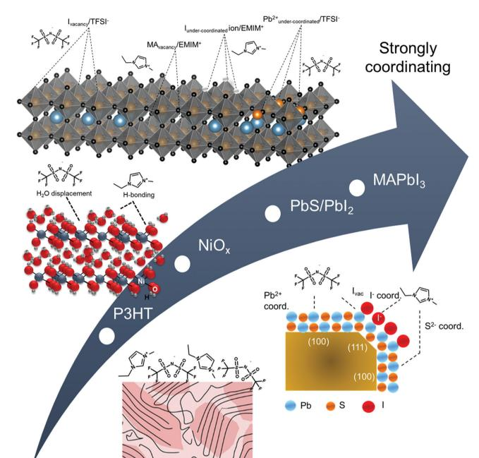
Fig. 5 Schematic representation of hypothesized near-surface interactions between ionic liquid and semiconductors from bottom to top: P3HT, NiO<sub>v</sub>, Pbl<sub>x</sub>-capped PbS quantum dots, and MAPbl<sub>3</sub>.
