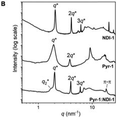
Fig. 1 (A) DSC trace (second heating and cooling cycle) of **Pyr-1:NDI-1**. A temperature ramp of 10 K min<sup>-1</sup> was used. Endothermic heat flows have a positive value. (B) 1D transmission scattering profiles of **Pyr-1:NDI-1** (bottom), **Pyr-1** (middle) and **NDI-1** (top) at room temperature.
