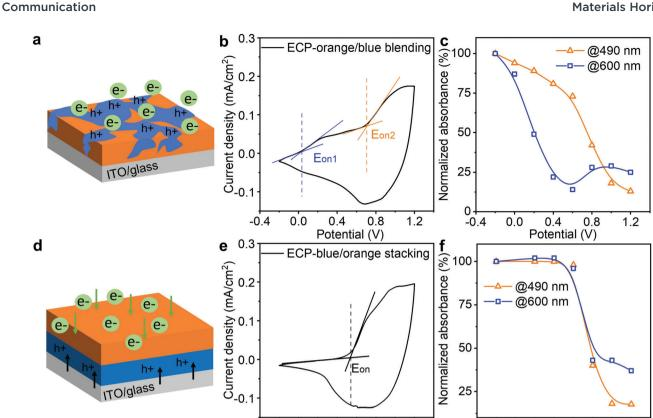
Fig. 4 Minimizing intermediate colors via unifying the electrochemical onset potentials. Electrochemical doping illustrations, cyclic voltammograms, and absorbance decrease for (a-c) ECP-orange/blue blending and (d-f) ECP-orange/blue stacking. e<sup>-</sup> and h<sup>+</sup> represent anions and holes, respectively.
