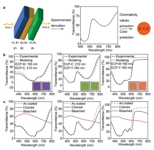
Fig. 2 Optical modeling-quided double-layer ECP stacking. (a) Workflow of the optical modeling. (b) Experimental vs. modeling spectra of the doublelayer ECPs consisting of various polymer thicknesses. The colors in the solid and dashed boxes are predicted by experimental and modeling spectra, respectively. (c) Spectroelectrochemistry of the double-layer ECPs.
