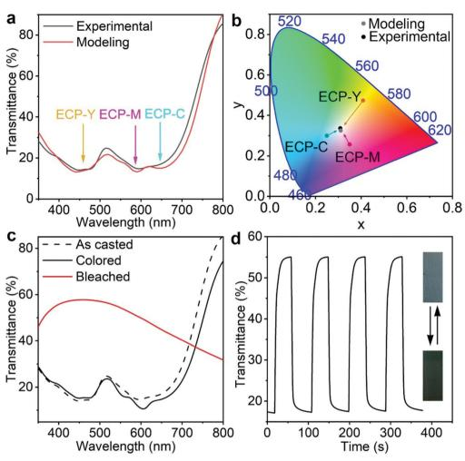
Fig. 3 Neutral grey electrochromic polymer from a triple-layer ECP. (a) Experimental vs. modeling spectra of the triple-layer ECP. (b) Chromaticity values extracted from the modeling and experimental spectra of the triple-layer ECP. The xy values of the constituent single-layer ECP-C, ECP-M, ECP-Y are also shown alongside. (c) Spectroelectrochemistry and (d) double potential step chronoabsorptometry of the triple-layer ECP.
