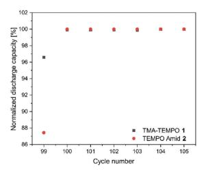
Fig. 1 Illustration of the discharge capacity of the first seven cycles of the TMA-TEMPO 1 and the amide 2 after the second hold time of 24 h. The capacity was normalized to the highest capacity in the shown interval. The first cycle showed a massively reduced discharge capacity.
