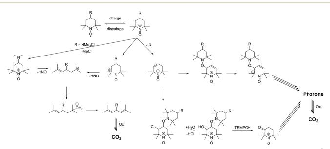
Scheme 1 Schematic representation of the proposed decomposition mechanism of TEMPO derivatives according to Ma et al. and Takata et al. 1.2
