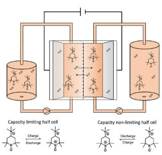
Fig. 2 Illustration of a symmetric TMA-TEMPO redox flow battery set up as well as the corresponding half-cell reaction.
