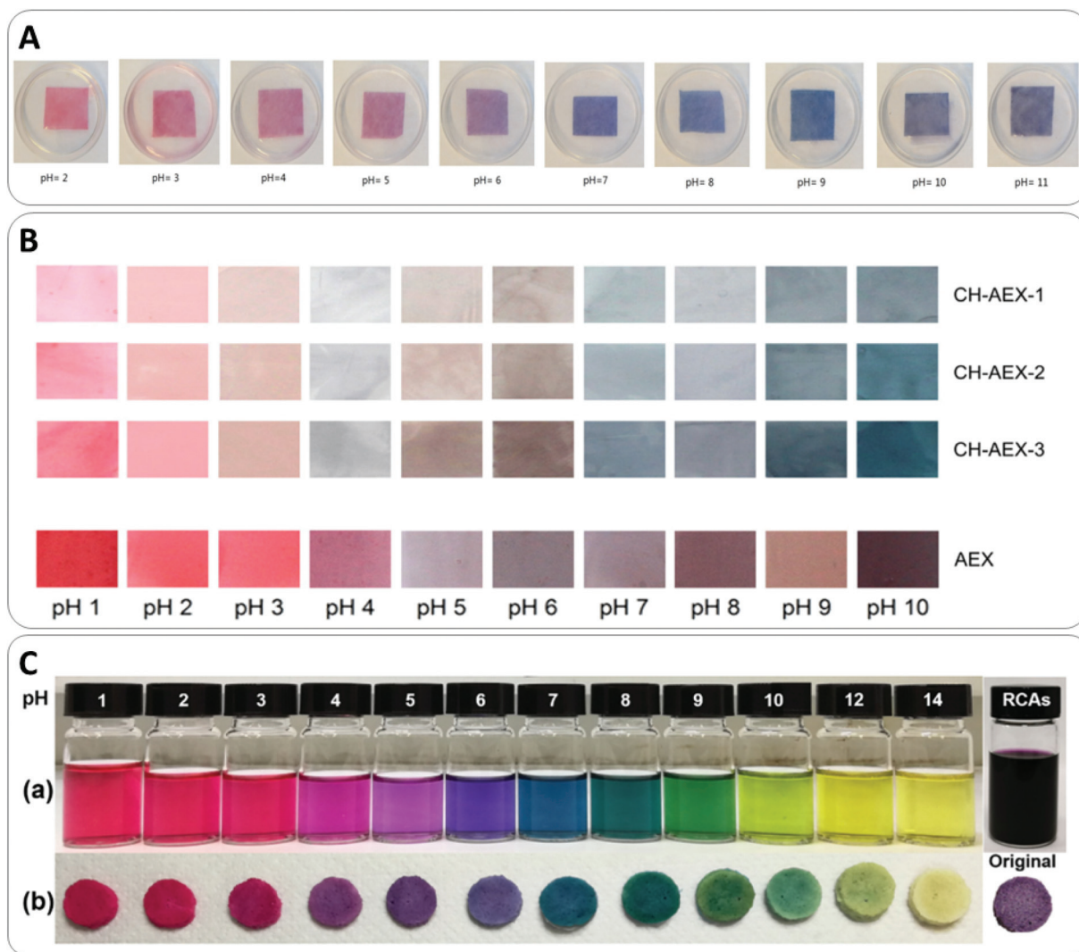
Fig. 4 Natural pH indicators. (A) Color changes for starch-paper films with carrot anthocyanins at different pH values (pH 2–11). Reprinted from M. M. Goodarzi, M. Moradi, H. Tajik, M. Forough, P. Ezati and B. Kuswandi, Development of an easy-to-use colorimetric pH label with starch and carrot anthocyanins for milk shelf life assessment, Int. J. Biol. Macromol. , 153, 240–247, Copyright (2020), with permission from Elsevier. (B) Color changes for chitosan films with different contents of black chokeberry pomace extract (AEX) immobilized in chitosan for colorimetric pH indicator film application, Food Packag. Shelf Life , 16, 185–193, Copyright (2018), with permission from Elsevier. (C) (a) Red cabbage anthocyanins (RCAs) solution response upon pH changes. (b) The PVA-PVP foam with MCC (thickness: 3.0 mm ± 0.2 mm, diameter: 14 mm) after dipping in solutions of different pH (in each case 10 ml for 3 min). Reprinted from J. Zia, G. Mancini, M. Bustreo, A. Zych, R. Donno, A. Athanassiou and D. Fragouli, Porous pH natural indicators for acidic and basic vapor sensing, Chem. Eng. J. , 403, 126373, Copyright (2021), with permission from Elsevier.
