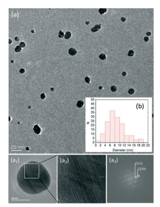
Fig. 1 TEM micrographs (a) and size distribution (b) of as-synthesized Ag-HEC NPs. TEM micrograph of Ag NPs at higher magnification (a1); close up showing lattice fringes (a2); and (a3) FFT indexed to cubic Ag (ICDD card no: 00-001-1167).
