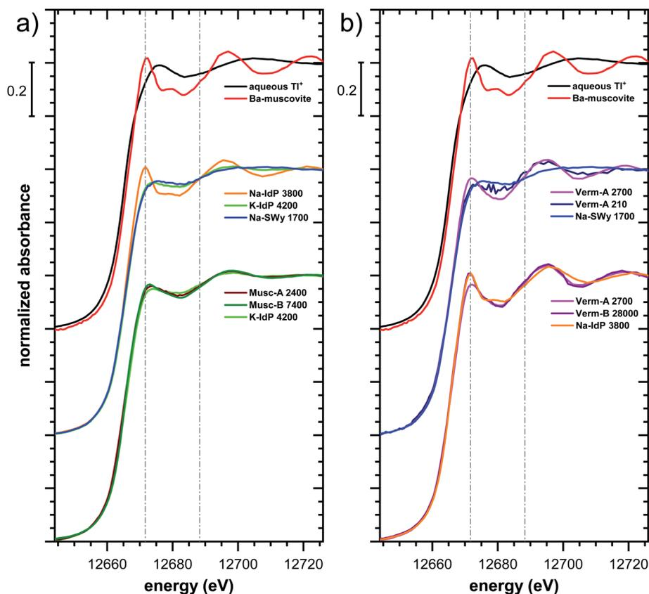
Fig. 5 Comparison of the Tl  $L_{III}$ -edge XANES spectra of selected Tl-loaded phyllosilicate samples. Numbers in spectra labels indicate the Tl loading of the respective phyllosilicate in  $\text{mg kg}^{-1}$ . Vertical lines serve to guide the eye. An enlarged version of figure focusing on post-edge oscillations is provided in Fig. S16.†
