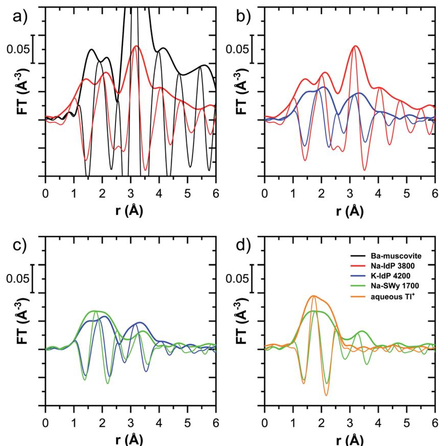
Fig. 6 Fourier-transformed  $k^2$ -weighted Tl  $L_{III}$ -edge EXAFS spectra of Tl-containing Ba-muscovite, Tl-loaded Na-IdP and K-IdP, Na-SWy and of aqueous  $Tl^+$ ; sequentially pair-wise compared (a–d; thick lines indicate magnitude, thin lines imaginary part). Numbers in sample names indicate the Tl loading of the phyllosilicates in  $mg\ kg^{-1}$ .
