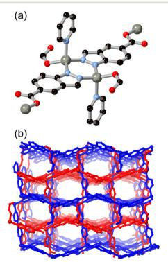
Fig. 5 (a) Coordination of the dianionic L5 linker to zinc ions in the presence of a dipyridyl co-ligand; (b) extended structure of the resulting MOF showing porosity retained between interpenetrating networks, coloured separately. Zinc atoms coloured grey.
