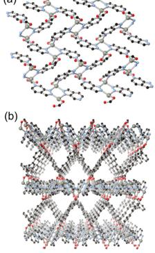
Fig. 6 (a) Structure of the two-dimensional Zn-L7 network formed in the presence of linking dicarboxylate co-linkers; (b) the extended structure of the ZnL7(bpdc) MOF showing triangular channels between dense zinc-azolate layers. Zinc atoms coloured grey.
