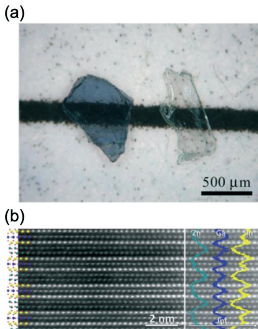
Fig. 16 (a) Single crystals of  $\text{In}_{1-x}\text{Ga}_{1+x}\text{O}_3(\text{ZnO})_{0.5}$  before (left) and after annealing (right). (b) HAADF image with crystal structure of  $(\text{InGaO}_3)_2\text{ZnO}$  overlaid (left) and extracted EDX line-scan profiles for In-L (yellow), Ga-K (blue) and Zn-K (cyan) as overlay (right). Panels (a and b) are reprinted with permission from ref. 68. © 2020 Elsevier.
