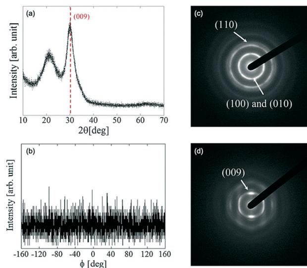
**Fig. 3** XRD measurement results for *c*-axis-aligned crystalline In-Ga-Zn-O: (a) out-of-plane XRD spectra and (b) in-plane ( $\phi$ -scan) XRD spectra ( $2\theta = 56^\circ$ ). (c) SAED diffraction pattern of CAAC-IGZO in the perpendicular direction, and (d) in the parallel direction. Panels (a–d) are reprinted with permission from ref. 10. © 2014 Society for Information Display.
