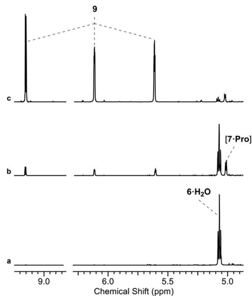
Fig. 2 Proline/phosphate co-catalysed reaction of glycolaldehyde phosphate and formaldehyde. <sup>1</sup>H NMR [400 MHz, noesyppprld, H<sub>2</sub>O/D<sub>2</sub>O (9 : 1)] spectra to show the reaction of glycolaldehyde phosphate (**6**, 100 mM) with formaldehyde (**8**, 100 mM) after 48 h at pH 7 and 40 °C: (a) in water; (b) with 50 mol% **L-Pro** in water; (c) with 50 mol% **L-Pro** in 500 mM phosphate.
