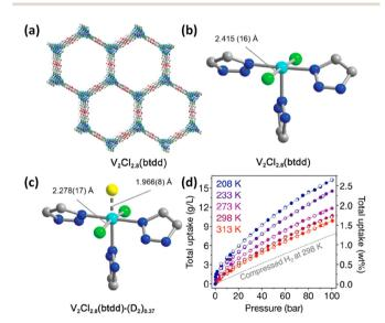
Fig. 6 (a) The 3D structure of  $V_2C_{12.8}$ (btdd) and the coordination environment of the V(II) centre in (b) the activated framework and (c) in the framework dosed with 0.75 equiv. of  $D_2$  molecules. (d) The high-pressure H<sub>2</sub> isotherm in the temperature range of 208-313 K. Reprinted with permission from ref. 56. Copyright 2021, American Chemical Society.
