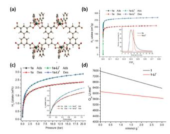
Fig. 9 (a) The partial structure of (Me<sub>2</sub>NH<sub>2</sub>)[In(L)] and comparison of (b) N<sub>2</sub> and (c) H<sub>2</sub> isotherms at 77 K and (d) H<sub>2</sub> adsorption heat for (Me<sub>2</sub>NH<sub>2</sub>)[In(L)] before and after Li<sup>+</sup> exchange. Reprinted with permission from ref. 70. Copyright 2008, Royal Society of Chemistry.
