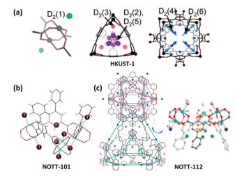
Fig. 5 D<sub>2</sub> binding sites in copper-multicarboxylate frameworks of (a) HKUST-1, (b) NOTT-101 and (c) NOTT-112 compounds as determined by the NPD experiment with D2 loadings of 4, 1.82 and 2.0 per copper ion, respectively. Reprinted with permission from ref. 42 and 43. Copyright 2006, and 2009-2010, American Chemical Society.
