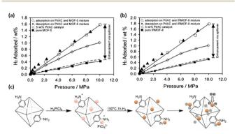
Fig. 10 Comparison of H<sub>2</sub> isotherms of (a) MOF-5 and (b) IRMOF-8 before and after Pt doping exhibiting significantly enhanced H2 storage capacities via the spillover effect. (c) Schematic representation of the synthetic route of Pt/aUiO that can dissociate dihydrogen to hydrogenate the organic linker. Reprinted with permission from ref. 80 and 81. Copyright 2006 and 2021, American Chemical Society.
