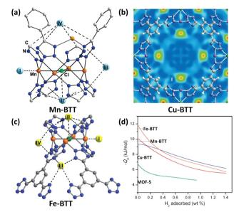
Fig. 4 D<sub>2</sub> binding sites in (a) Mn-BTT, (b) Cu-BTT and (c) Fe-BTT compounds as determined by the NPD experiment with the D2 loadings of 12, 30 and 20 per formula unit, respectively, and (d) comparison of their H2 adsorption heats. Reprinted with permission from ref. 36, 38 and 39. Copyright 2006, American Chemical Society; Copyright 2007, Wiley; Copyright 2010, Royal Society of Chemistry.
