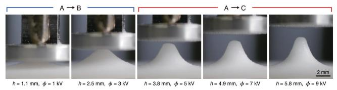
Fig. 10 Particle raft deformation at the regime boundary of Fig. 2(c). The upheaved raft touches the electrode at low h and  $\phi$  (boundary of regimes A and B). On the other hand, at high h and  $\phi$  (boundary of regimes A and C), the rafts stop without touching the electrode.
