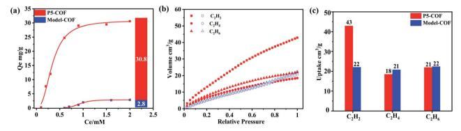
Fig. 2 (a) Langmuir adsorption isotherms of paraquat by P5-COF and Model-COF. Inset: the comparison of the paraquat adsorption capacity of P5-COF and Model-COF; (b) gas adsorption isotherms of P5-COF (red) and Model-COF (blue) at 273 K; (c) comparison of gas adsorption uptakes of P5-COF and Model-COF at 273 K.
