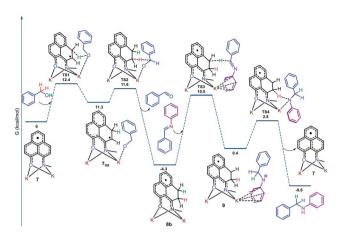
**Fig. 1** Energy profile diagram along the reaction coordinate for the catalytic *N*-alkylation, obtained from DFT calculation. Only one isomer is represented for the sake of simplicity.
