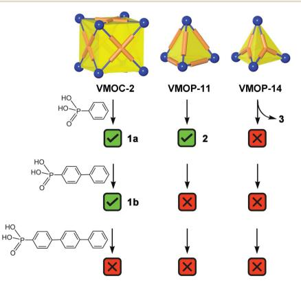
Scheme 1 Summary of the outcome of endohedral functionalization with organophosphonic acids with increasingly lengthy phenyl tails. The vertex directing units (blue spheres) are  $\{V_6S\}$  SBUs and the linker groups (orange tubes) represent ditopic and polytopic carboxylate ligands.
