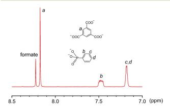
Fig. 5 The <sup>1</sup>H NMR spectrum of a base-digested sample of 3 (400 MHz, NaOD/D2O, 293 K).
